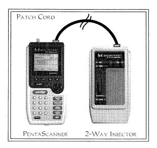
From the PentaScanner Ready! screen, press; then select Injector Status to display 2-Way Injector information on the PentaScanner screen:
