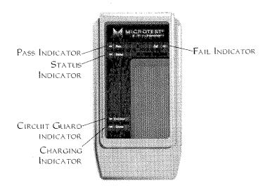
The 2-Way Injector features LED indicators and an audible tone generator. Each is described in the following sections:
