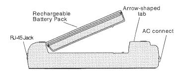
The 2-Way Injector is powered by a rechargeable, recyclable Nickel Cadmium (Ni-Cd) battery pack. Under various state and local laws, it may be illegal to dispose of this battery pack into the municipal waste stream. Check with your local solid waste officials for details in your area for recycling options or proper disposal.
