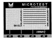
➤ Note: Straight through wiring is the expected case.
